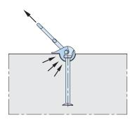
Consequently there is no reduction in load bearing capacity to account for diagonal loading in large surface elements. For example; as is standard for sleeve anchors. Additional reinforcement is not required.
