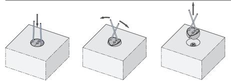
There are two holes in the recess former to help prise it out of the hardened concrete. Two reinforcement bars can be inserted in these holes and crossed against each other to open and remove the recess former. Excess concrete should be removed.
