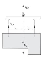
The load's centre of gravity will always stabilise verticality under the crane hook. Load distribution in non-symmetrically installed anchors when using a spreader beam is calculated as below:
