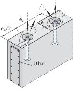
Required reinforcement 1 – 3. Reinforcement 4 only with diagonal pull  $\rightarrow$  see table on page 22 "reinforcement in walls".
