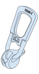
Allowable loads for each particular case can be found in the respective tables. In general the safety regulations in the country of use are to be observed, in particular those for the use of cranes and lifting equipment. The DEHA Universal head lifting link is used for lifting and transporting precast concrete elements with cast in spherical head anchors. The universal head lifting link is a manual-release link. The universal head links currently available are Chrom-6-free zinc galvanized.
