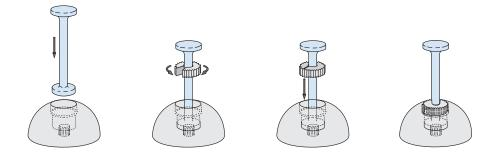
Slide the rubber grommet onto the anchor and press both into the hole in the steel recess former. If necessary, grease before use. Ensure the anchor is securely fitted and tied in place when the concrete is being poured.
