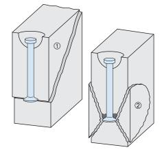
0 Expected failure if anchor load is too high 0 Blow-out failure only in very thin elements
