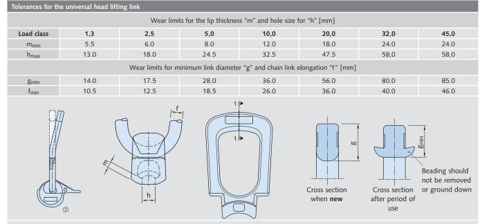
① It is prohibited to rebend any element damaged by misuse. Discard the universal head lifting link if there is any significant bending.
