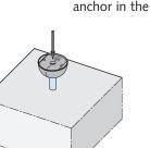
make a hole by removing a small amount of concrete with a trowel, place the recess former with the anchor in the hole.
