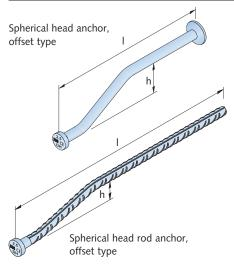
The offset spherical head anchor only differs from the standard spherical head anchor as it is bent. The special shape allows the anchor to be used in multi-layer elements. In special cases the offset spherical head anchor can be used in thin shell elements, for example in precast garages or sandwich panels.
