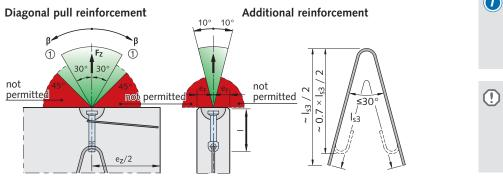
Required reinforcement a only with diagonal pull → see table on page 22 "reinforcement in walls".
