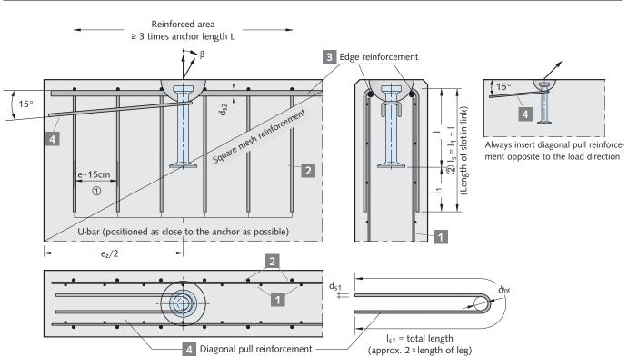
Additional reinforcement when using the spherical head anchors in wall elements
