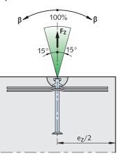
Required reinforcement 1 - 3. Pitching reinforcement is used instead of diagonal pull reinforcement → see table on page 22 "reinforcement in walls".
