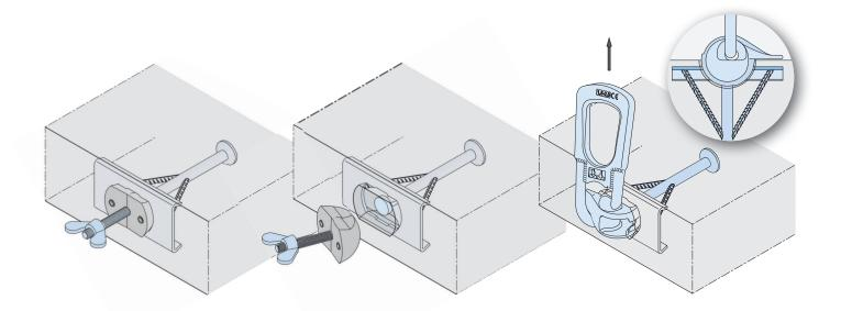
Insert the DEHA KKT Spherical head lifting anchor into the narrow rubber recess former and insert both in the hole in the pitching plate. The narrow recess former and the attached metal parts are fixed to the formwork.
