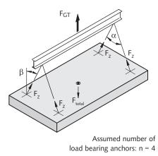
A perfect static weight distribution can be achieved using a spreader beam which avoids diagonal pull.
