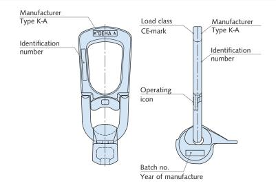
The application identifier K-A denotes that the universal head lifting link can be used for the following two DEHA Lifting anchor systems:
