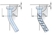
After installation the anchor head is near the centre axis of gravity. To ensure safe load anchorage the anchor foot is located in the centre of the support layer. This allows near vertical lifting and installation.
