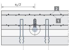
Additional sandwich anchor pins positioned around the anchor can be beneficial
